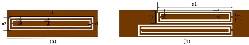
Figure 1. Layout of the CODMS cell and proposed two cells structure (a) parameters of one cell: a_1 = 15 mm, a_2 = 1.8 mm, a_3 = 0.3 mm, w = 0.2 mm. x_1 = 0.25 mm, (b) parameters of below cell: a_1 = 15 mm, a_2 = 1.8 mm, a_3 = 0.3 mm, w = 0.2 mm, x_1 = 0.25 mm; parameters of top cell: a_1 = 11.9 , a_2 = 2 , a_3 = 0.3 mm, w = 0.2 mm, x_1 = 0.2 mm.
